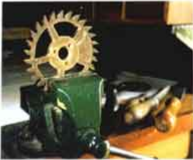
The escape wheel - most of the teeth were missing from the original so a replica was made.
