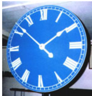
The dial - this is made of rolled brass sheet and engraved with Roman numerals.
